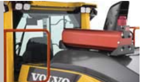
Fire suppression system
