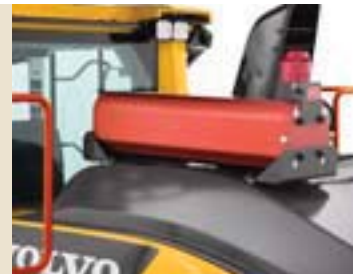
Fire suppression system
