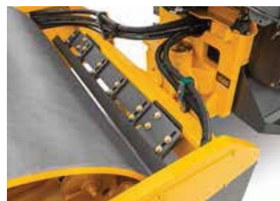
Inside drum scraper
